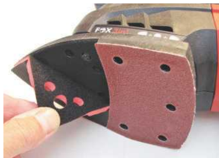
The pads are secured with hook & loop fixings...
